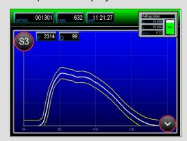
Dynamic envelope monitoring is applied to all channels. Up to 16 channels can be monitored.
