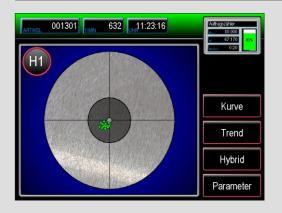
The new **Hybrid***master* set-up assistant for presses shows on a target screen if punch and die side tools are properly aligned when used in conjunction with our hybrid sensors (patent applied for).
