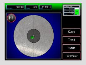
The new **Hybrid**master set-up assistant for presses shows on a target screen if punch and die side tools are properly aligned when used in conjunction with our hybrid sensors (patent applied for).
