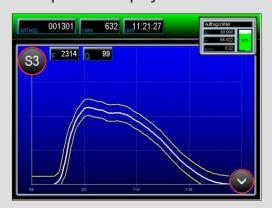
Dynamic envelope monitoring is applied to all channels. Up to 16 channels can be monitored.
