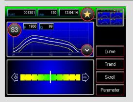
The **SK**ROLL*master*® die match indicator assists operators in aligning thread roll dies quicker, more precisely, and more efficiently.
