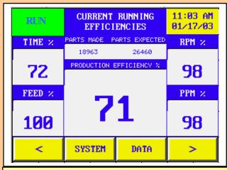
The Current Running Efficiencies Screen displays up to the minute percentage rates for Time, Feed Rate, RPM, PPM, and Production. Time and Production Efficiency reset each shift. Other efficiency screens are included.
