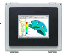
touch-screen interfaces that are now available in 4", 6", and 8" sizes. These screens display real-time production totals, machine efficiency, and accumulated machine uptime and downtime. The new 8" screen provides twice the previous resolution, so more information can be shown on each screen, resulting in a better overview of machine status at a glance.
