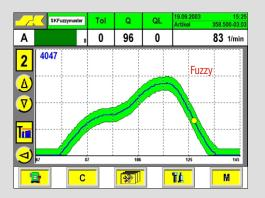
The new SKFuzzymaster-Software ensures that the envelope width is always set so that the current process is perfectly monitored.
