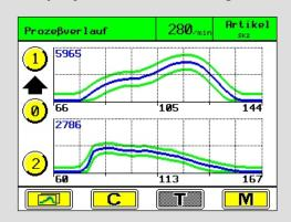
Dynamic enveloping with visual presentation of force curves and current envelope limits (single and dual channel display).
