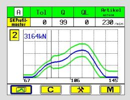
SKProfilemaster represents the next generation of force monitoring: the new "profile enveloping technique" by SK improves the monitoring performance even more. Sensitive where needed, and less sensitive during unstable forming phases. SKProfilemaster ensures optimum sensitivity and maximum productivity by avoiding nuisance machine stoppages.
