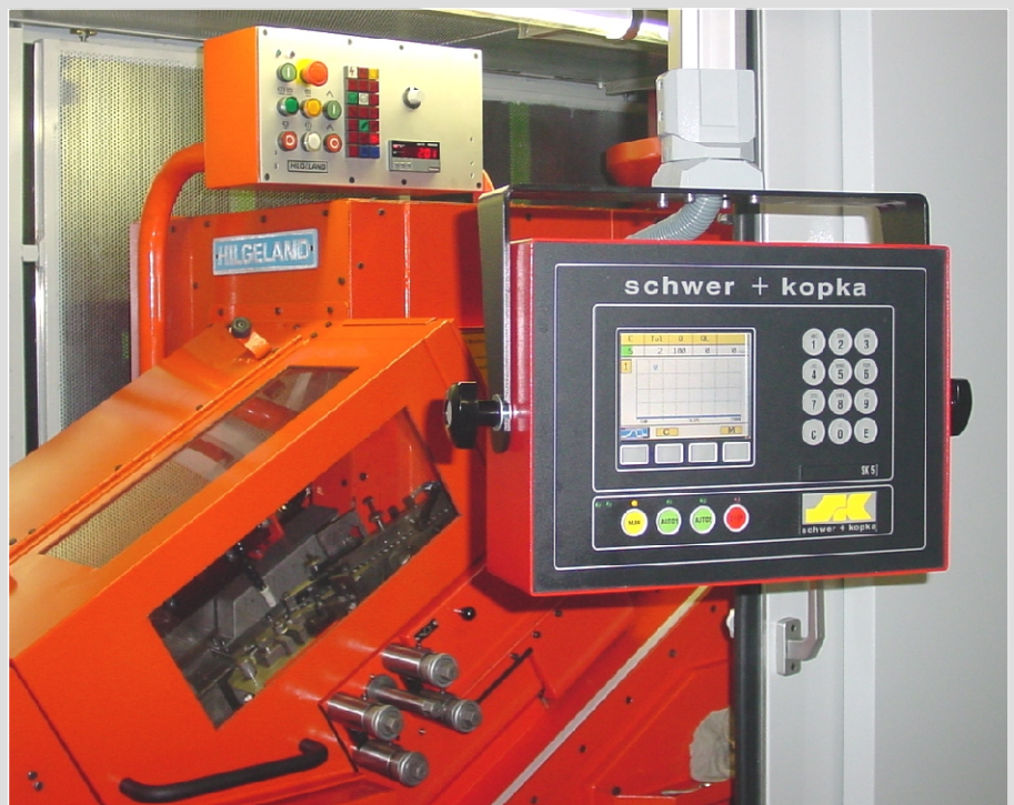
Process monitor type SK 2 with SKSinglemaster in operation on a thread roller
