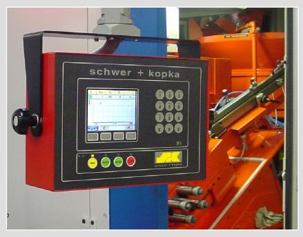
The SKROLLmaster® "freeze-function" is available for the IMPAX/SK 2 and 5 (above), the IMPAX/SK 100, the PC-based models IMPAX/SK 4 and IMPAX/SK 7, and the integrated version IMPAX/SK-bbx on new machines with PC-controls.
