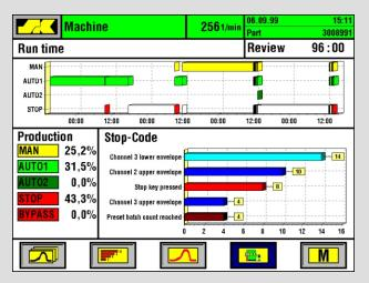
Machine run time chart shows uptime vs. downtime, error frequency, and machine efficiency.
