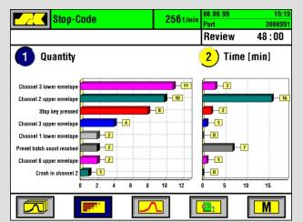
Error statistics show the distribution of stop codes and resulting accumulated down time.
