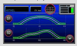
Dynamic envelope monitoring is applied to all channels. Up to 16 channels can be monitored.
