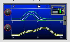
Dynamic envelope monitoring is applied to all channels. Up to 8 channels can be monitored with 2 being displayed simultaneously.
