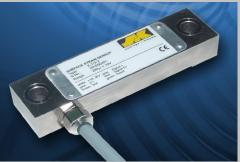
The X-flex sensor is a strain sensor and is usually attached to the frame of a machine to protect the machine from an overload condition. The surface strain (tension or compression) is directly related to machine load, for example, on presses.
