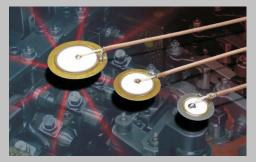
Diskflex sensors are significanly less expensive than the Superflex sensors and are epoxied into areas for best signal pickup. They have been used in wedges, backing plates, feed stops, and even embedded into tool holders. Many sizes are available from 8.9mm to 50mm.
