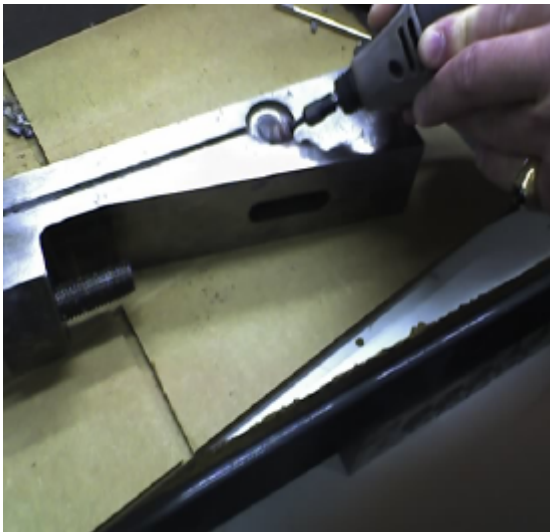
1) Roughen any smooth surfaces for better adhesion of the new epoxy.
