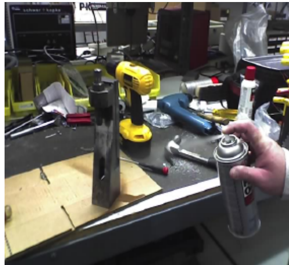
2) Clean out sensor and wire pocket to remove all grease and debris.
