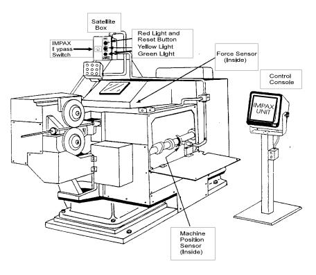
The **Satellite Box** is the junction for all the controls and components on the machine. The **Reset Button** is the only operator control. The **Bypass Key Switch**, operated by the Supervisor's Key, disables the relay which stops the machine and its accessories, but has no other effect on operation. Note: There is no machine protection when the IMPAX 500 is in Bypass mode.
