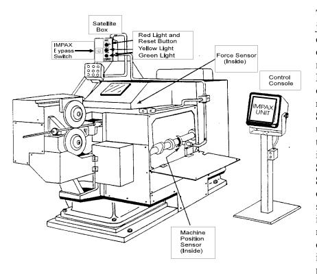
The **Satellite Box** is the junction for all the controls and components on the machine. The **Reset Button** is the only operator control. The red, yellow, and green Status Lights indicate the mode of operation that the IMPAX unit is in. The **Bypass Key** Switch, operated by the Supervisor's Key, disables the relay which stops the machine and its accessories, but has no other effect on operation. Note: There is no machine protection when the
